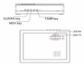
C. When LED-RF and LED-FS flash alternately after they light 1sec., it means the data exchange is completed. Please touch TAMP key for exit.
